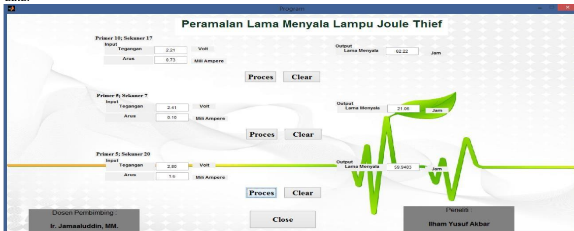
Figure 9. Forecasting Data Collection on Three Different Joule Thief Circuits via Matlab GUI
