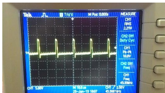
Figure 8. Display Result of Joule Thief Output Voltage Signal on Oscilloscope
